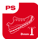
PS Non-metallic perforation- resistant inserts and insoles
